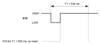
When the condition is met that a LOW level is applied across the control input X10 for at least T1 = 530 ms, disturbing pulses will not cause a RESET of the residual current monitoring module.
