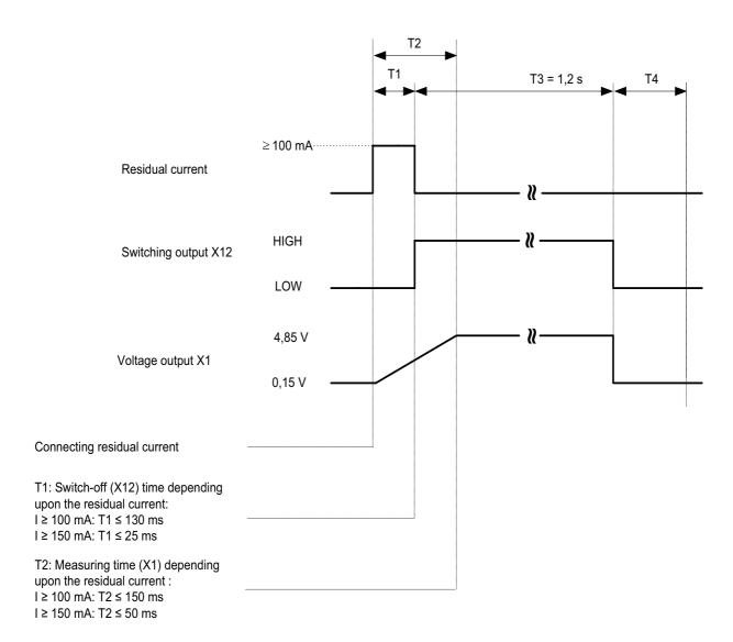
If the residual current exceeds the measuring range (residual current ≥ 100mA), the residual current monitoring module RCMA278P-S will switch the Open-Collector output to HIGH once the measuring time T1 has elapsed.
