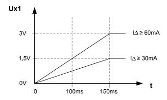
Switching times at the switching output X12:
