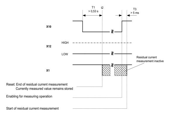
A RESET of the residual current monitoring module RCMA278P-S can be carried out at any time via the control input X10. In this case, the residual current measurement process has to be interrupted.
